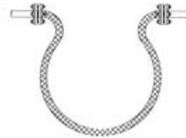
Case 3 - The horizontal movement of a hose loop (Figure 5) must be directed in the same plane as the loop (Figure 6). Movement out-of-the-plane or with the loop offset (Figure 7) will result in unnecessary torsion on the hose. The torsional stress will result in hose failure
