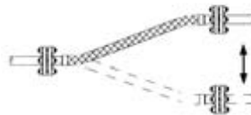
Case 5 - A hose loop with elbows (Figure 11) is more Suited for vertical movement than a straight hose (Figure 12). The vertical movement will cause bending stresses at the hose ends, resulting in a hose failure.
