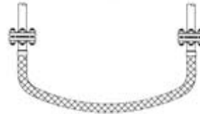
Figure 2 Case 2 - Avoid bending the hose at the end Connections (Figure 4). Install 90° pipe Elbows in horizontal pipe runs with hose Loops (Figure 3). The proper live length and bend radius must be taken into account as in Case 1 (Figure 1).
